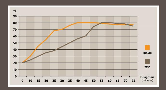
The graph above shows the comparison in temperture rise between the new Ecoboiler (EB16HE) and the previous Stratford model (TF50).
