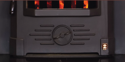
Spin Valve controls primary combustion air supply, with intake slot for convection heating
